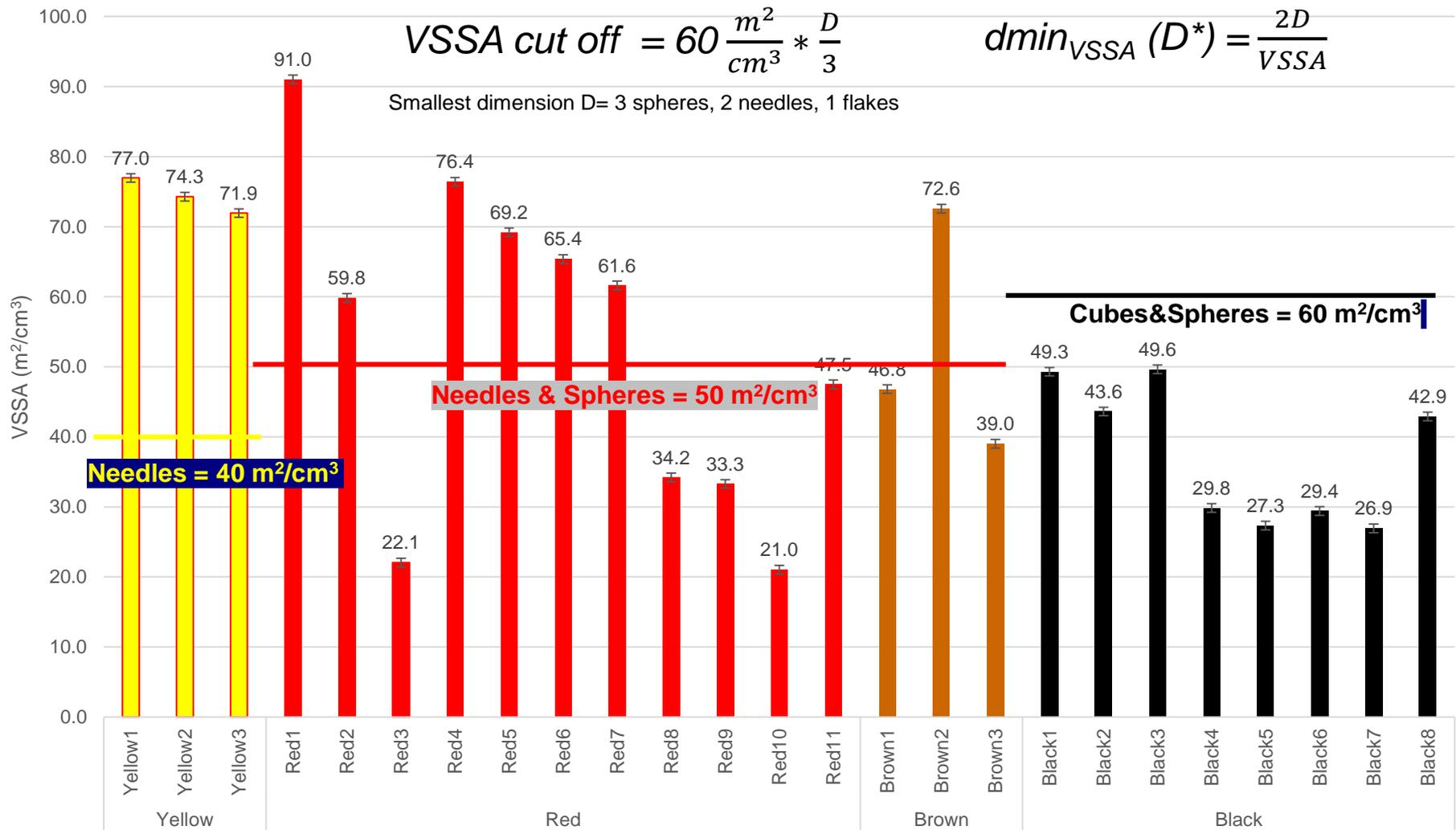
According to DIN ISO 9277, samples are heated up to 180°C in 30 min and left at this temperature for one hour before determination of the SSA under Nitrogen at 5 different pressure ratios: 0,1 – 0,15 – 0,2 – 0,25 – 0,3.
