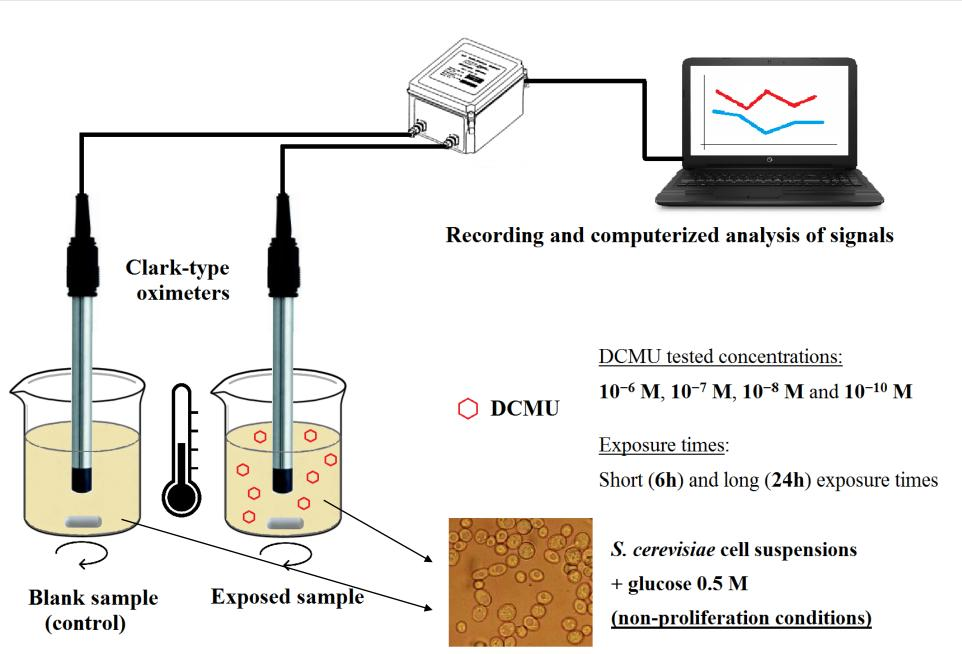
All tests were performed in **controlled** and **constant** conditions of temperature  $(25.0 \pm 0.1 \, ^{\circ}\text{C})$  and agitation (stirring speed: 200 rpm)
