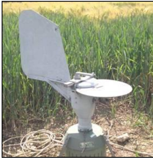
Spore traps - air particles impacted onto waxed tape
