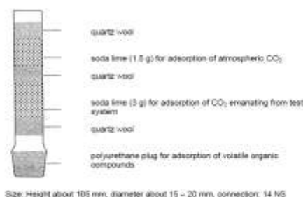
Figure B.8.2.1.2.2._CA-12: The Test vessel type A used in the experiment (copied from the study report).
