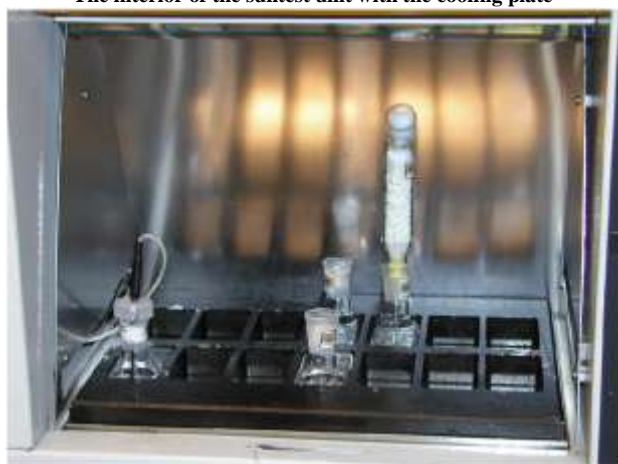
The interior of the suntest unit with the cooling plate
