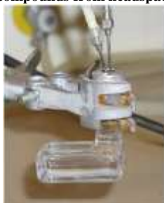
Sealed test vessel with injection needles used to remove volatile compounds from headspace
