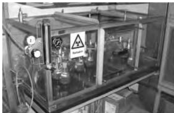
Figure B.8.1.1.1.2._CA-13: The anaerobic incubation chamber used in the experiment (copied from the study report).
