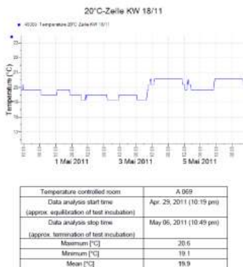
Figure B.8.1.2.1.2._CA-18: The graphical results of the monitoring of the temperature during the study (copied from the study report).
