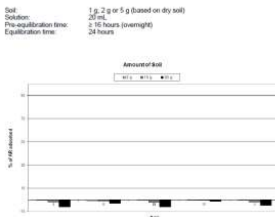
Figure B.8.1.2.1.2._CA-32: The graphical results of the determination of the appropriate soil:solution ratio – amount of Trifluoroacetic acid (TFA) adsorbed onto soil (copied from the study report).
