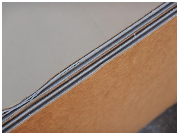
**PHOTOGRAPH 2** Folding floor of pressed cardboard, thickness 1.5 cm in two layers.
