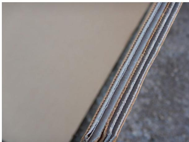
**PHOTOGRAPH 1** Folding floor of pressed cardboard, thickness 3 cm in three layers.
